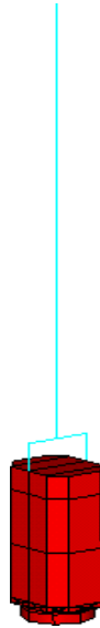
Fig. 4. General view of the finite-element model of the container with fresh fuel
